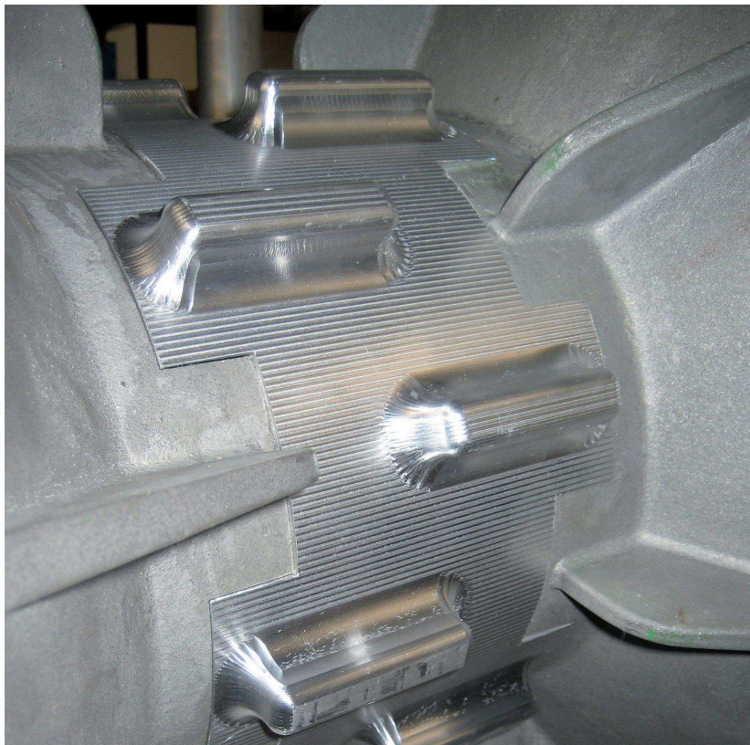
ADAPTATION: Isabelle Blancard of VirHydro said that the haulers have been modified for French Guyana, with the drums made wider to allow them to haul acoupa without damaging the fish
